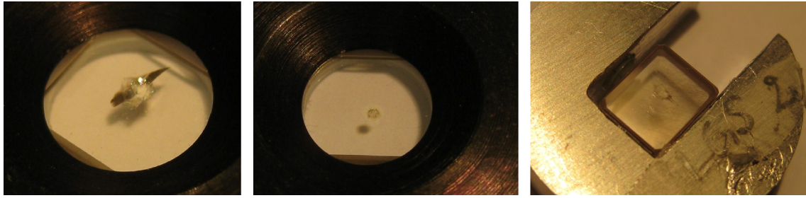
Fig. 1. Surface damage in sample #1 (left), sample #2 (middle) and old LGS sample (right).
