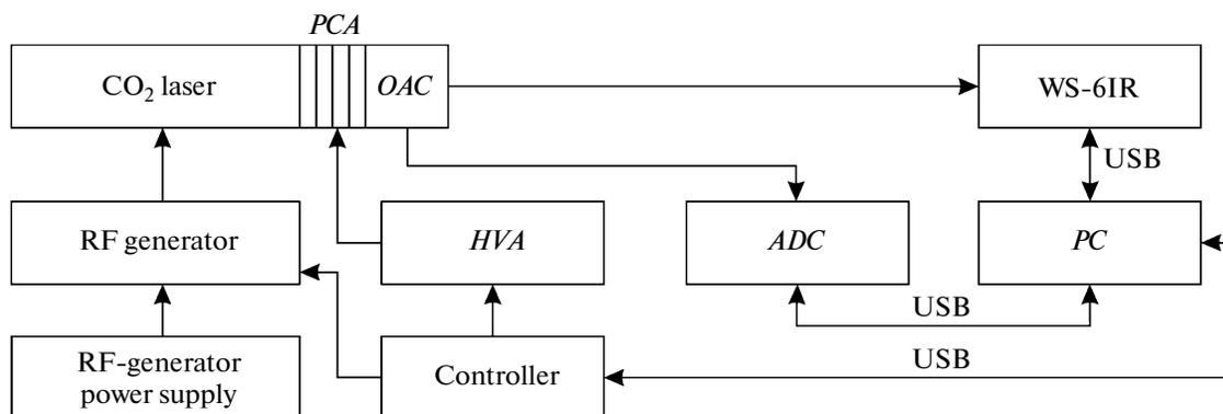
**Fig. 1.** Structural diagram of the instrument: (*OAC*) optoacoustic detector, (*HVA*) high-voltage amplifier, (*PCA*) piezoceramic actuator, (*ADC*) analog-to-digital converter, and (*PC*) personal computer.
