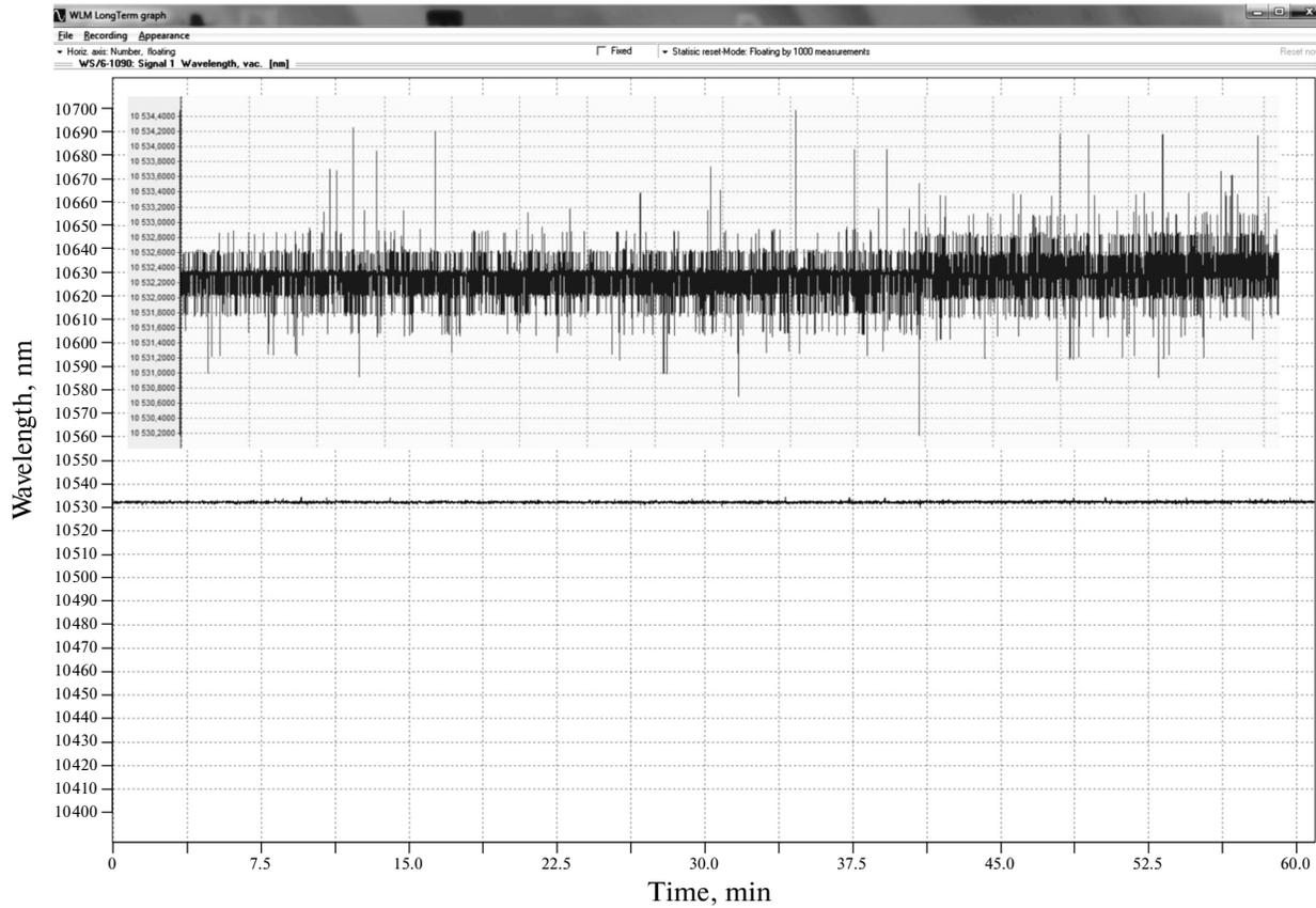
Fig. 4. WS-6IR signal during laser operation in the 10P(14)-line stabilization mode.
