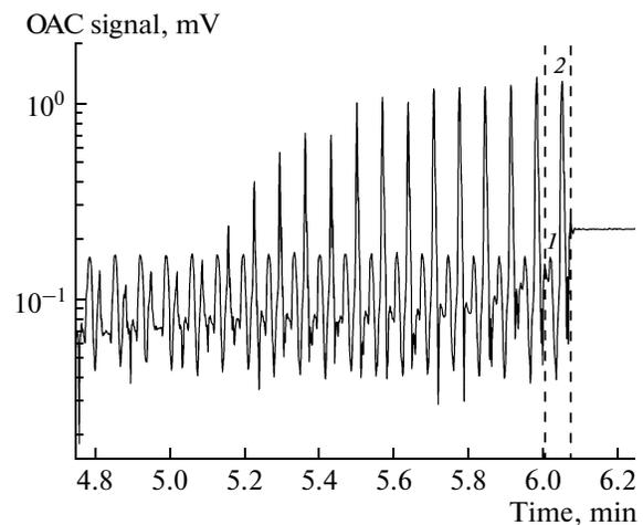
Fig. 3. OAC signal during operation of the 10P(14)-line searching algorithm. Dashed lines denote the time interval of one laser-contour tuning cycle.
