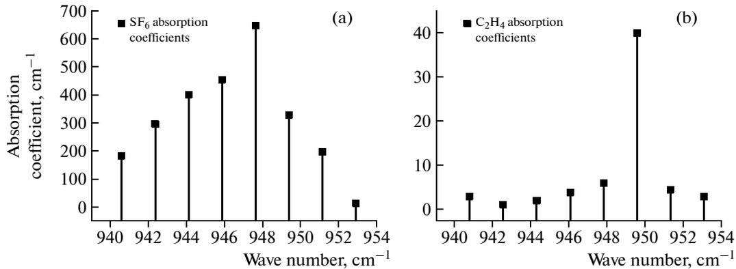
Fig. 2. (a)  $\text{SF}_6$  and (b)  $\text{C}_2\text{H}_4$  absorption spectra at the  $\text{CO}_2$ -laser emission lines in the range of 943.9–961.5  $\text{cm}^{-1}$ .
