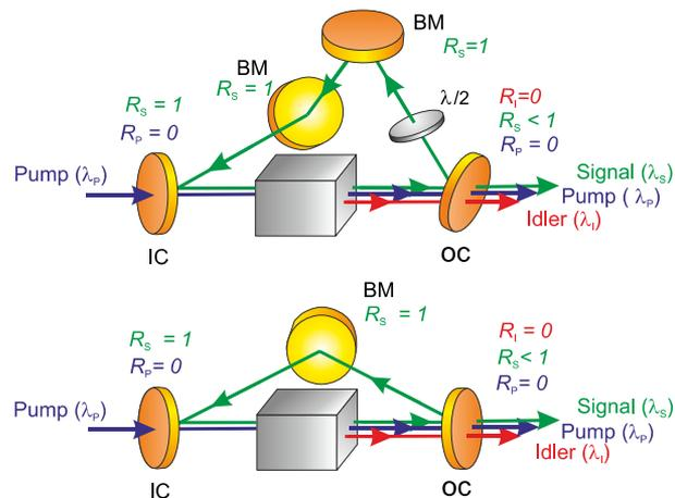
Fig. 2. RISTRA (top) and planar ring (bottom) OPO cavities investigated. IC, input coupler; OC, output coupler; BM, bending mirror; R, reflectivity.
