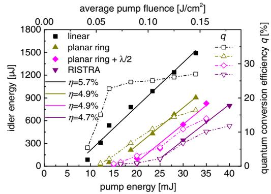
Fig. 6. Idler energy and quantum conversion efficiency obtained with HGS #3 and  $D_p = 5.35$  mm in linear, planar ring, and RISTRA cavities. An additional case of a planar ring cavity with a half-wave plate is also included.
