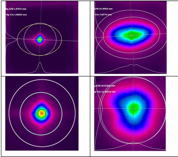
Fig. 10. Idler beam profiles with the planar ring (top) and RISTRA (bottom) cavities recorded at 19 cm (left) and 56/63 cm (right) from OC at large ( $D_p = 5.35$  mm) pump diameter. The pump energy is 35 mJ for the planar ring and 42 mJ for the RISTRA cavity.
