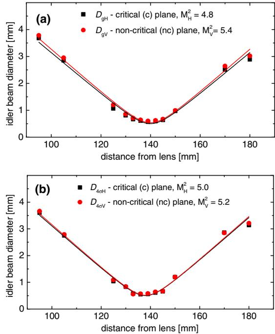
Fig. 11.  $M^2$  fits (lines) to the experimental idler beam widths in terms of (a) Gaussian and (b) second-moment diameters in the two planes obtained with the RISTRA cavity at large ( $D_p = 5.35$  mm) pump diameter and 42 mJ pump energy.
