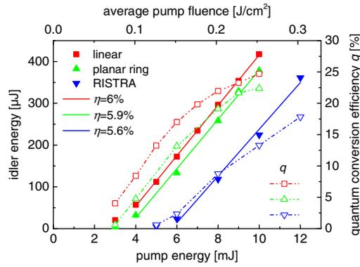
Fig. 5. Idler energy and quantum conversion efficiency obtained with HGS #2 and  $D_p = 2.25$  mm in linear, planar ring, and RISTRA cavities.
