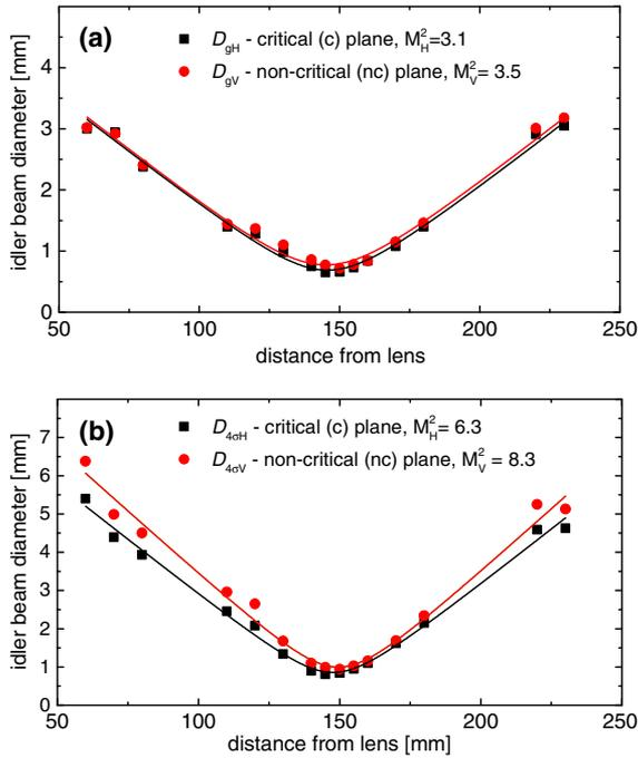
Fig. 8.  $M^2$  fits (lines) to the experimental idler beam widths in terms of (a) Gaussian and (b) second-moment diameters in the two planes obtained with the RISTRA cavity at small ( $D_p = 2.25$  mm) pump diameter and 12 mJ pump energy.
