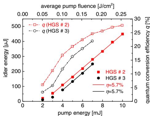
Fig. 4. Idler energy and quantum conversion efficiency obtained with HGS #2 and HGS #3 in a short linear OPO cavity.
