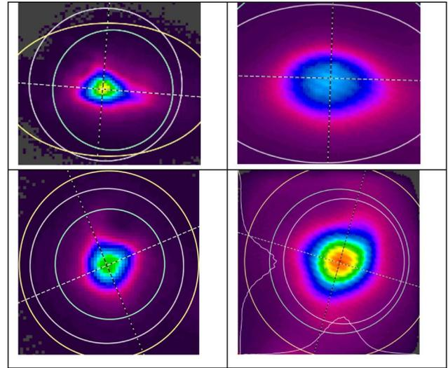
Fig. 7. Idler beam profiles with the planar ring (top) and RISTRA (bottom) cavities recorded at 14 cm (left) and 42 cm (right) from OC at small ( $D_p = 2.25$  mm) pump diameter. The pump energy is 9 mJ for the planar ring and 12 mJ for the RISTRA cavity.
