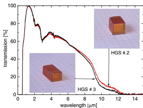
Fig. 3. Measured unpolarized transmission of the two HGS samples used.
