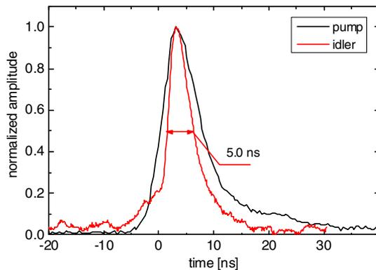
Fig. 9. Idler pulse temporal profile obtained at maximum energy with the RISTRA cavity using HGS #2 with a pump diameter of  $D_p = 2.25$  mm.
