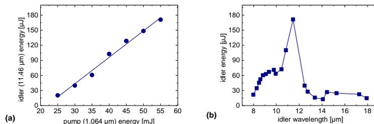
Fig. 2. Idler  $I_2$  energy of the AGSe SRO at 11.46  $\mu\text{m}$  (normal incidence,  $\theta=51.3^\circ$ ) vs. pump  $P_1$  energy at 1.064  $\mu\text{m}$  (a), and angle tuning of the AGSe SRO in the mid-IR at a pump energy of 55 mJ at 1.064  $\mu\text{m}$  (b).
