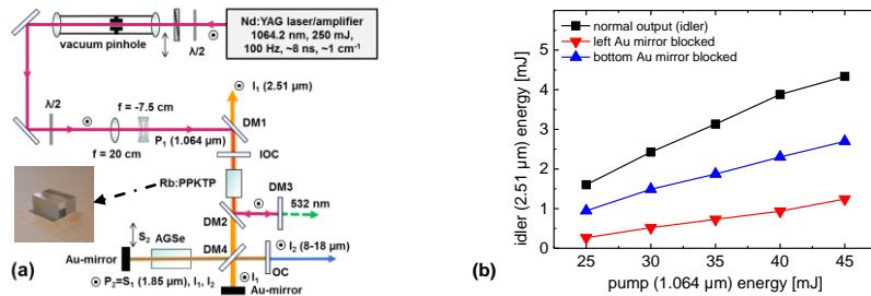
Fig. 1. Schematic of the intracavity pumped, cascaded AGSe OPO (a), and performance of the first stage (idler  $I_1$ ) without the AGSe crystal (b).
