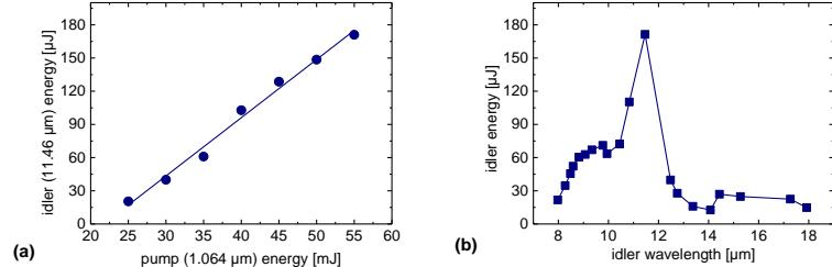
Fig. 2. Idler  $I_2$  energy of the AGSe SRO at  $11.46\text{ }\mu\text{m}$  (normal incidence,  $\theta=51.3^\circ$ ) vs. pump  $P_1$  energy at  $1.064\text{ }\mu\text{m}$  (a), and angle tuning of the AGSe SRO in the mid-IR at a pump energy of  $55\text{ mJ}$  at  $1.064\text{ }\mu\text{m}$  (b).
